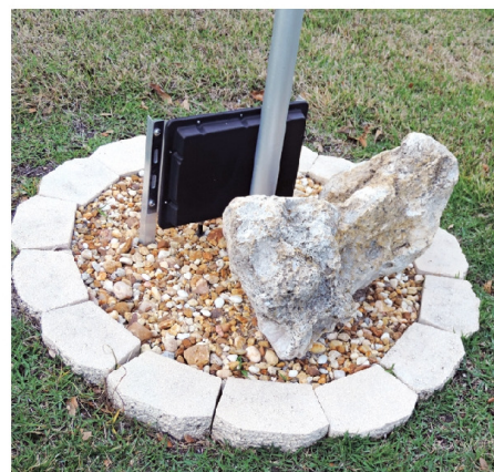
Figure 2 — The antenna tuner unit is the black box at the base of the flagpole. [Jeanette Ellis, NP2C, photo]
