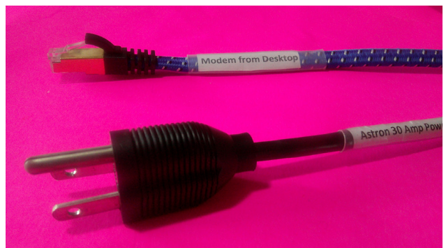
Figure 2 — Wire labels sealed with clear heat-shrink tubing. [Steve Mollman, KD9HL, photo]
