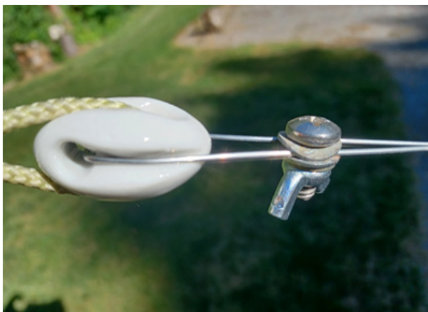
Figure 4 — A screw and two flat washers keep the dipole wires from twisting. [Paul Conaway, KD2DO, photo]
