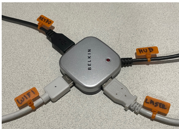
Figure 3 — Tagged zip ties being used as wire labels on the USB hub. [Ray Fallen, ND8L, photo]
