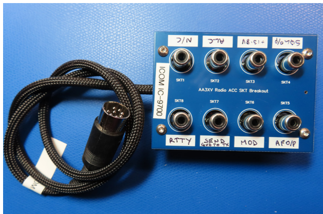
Figure 1 — A completed breakout board interface. [Kevin Jackson, AA3XV, photo]
