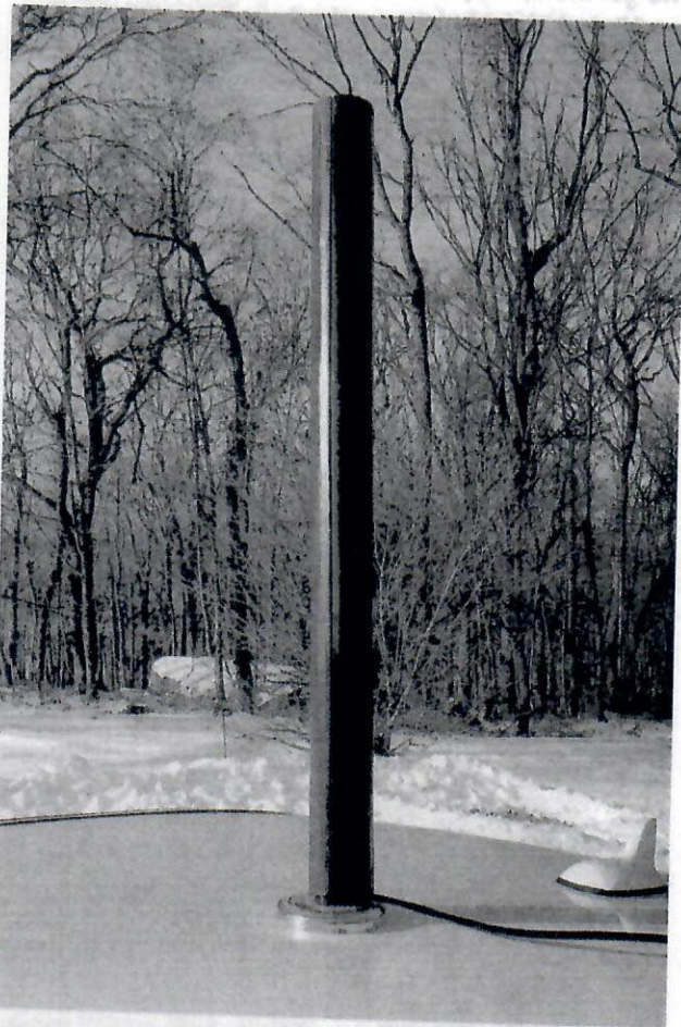
Figure 1 — The carbon fiber tube placed over Jay Kolinsky's, NE2Q, magnetic mount antenna on his car.
