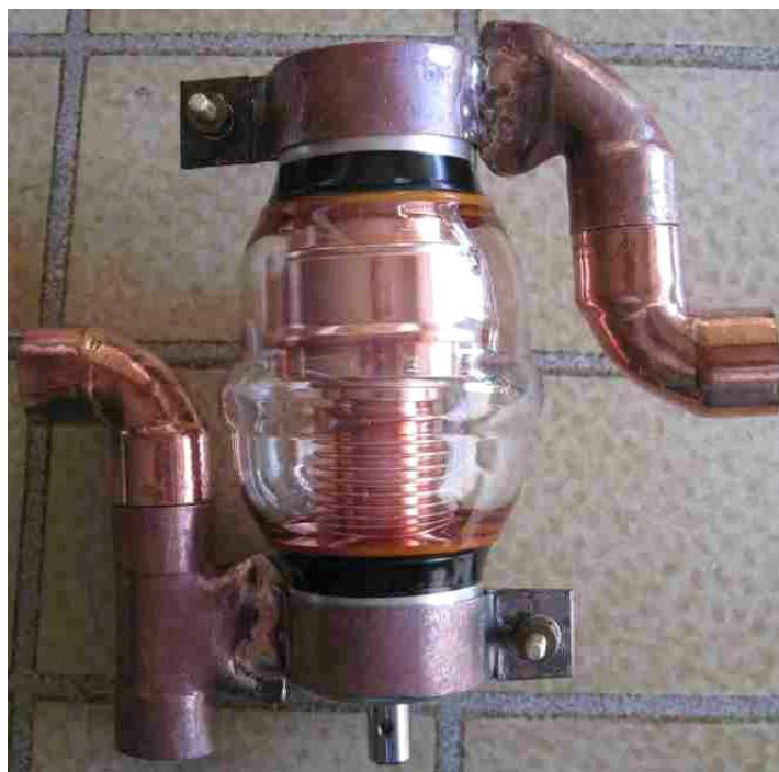
Figure 16 Homebrew capacitor clamps with silver-soldered copper fittings
