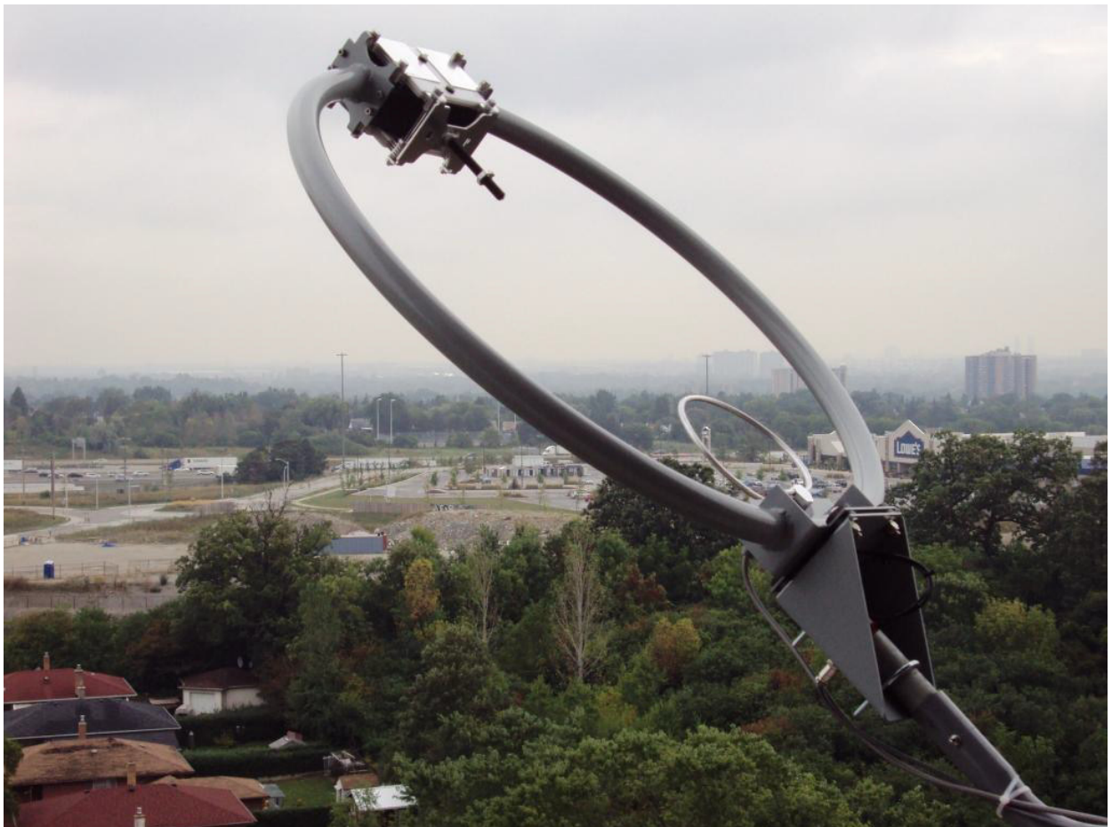
Figure 22 An MLA deployment on elevated condominium balcony
