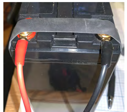
Fig. 2 Elastic band covers most of the exposed screw terminals
