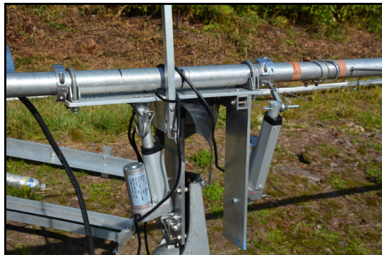
Elevation mechanism for the 2 meter antenna, which was used for the EME try.
