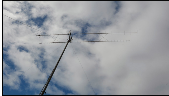
This photograph shows the 222 MHz and 432 MHz antennas at 50 feet on the AB-577.
