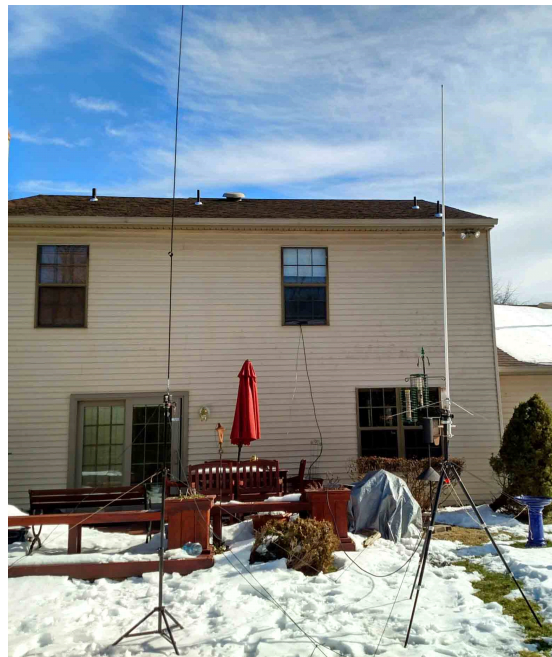
My Temporary Antenna Setup with the 6M Vertical on the Left and the 2M/70cm Vertical on the Right.
