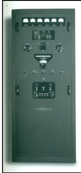
Figure 4, Collins KW-1. 1 KW CW, AM and NBFM Transmitter with VFO Exciter. circa 1950.
