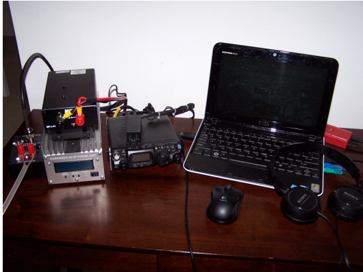
Figure 2, Up-graded vacation station with 50 watts output for 40 to 10 meter operation.
