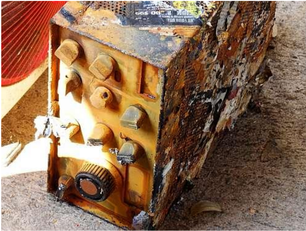
That's a Drake T-4XC under the murk and mud, while trophies and plaques were not spared flood damage.
