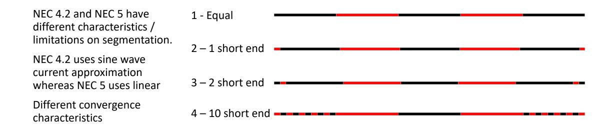
Model a half-wave dipole with different wire radius with respect to wavelength using different numbers of segments and for NEC 5 investigate use of short end segments to improve convergence with fewer segments.
