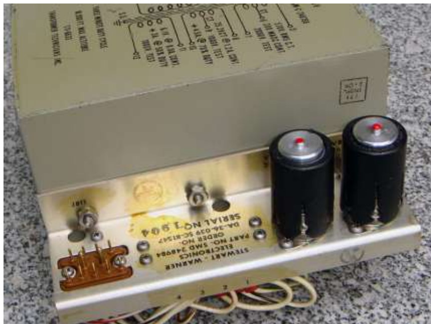
Fig. 2 Power supply chassis equipped with a pair of 26Z5W replacement modules with short height IERC tube shields (TR6-6015B)
