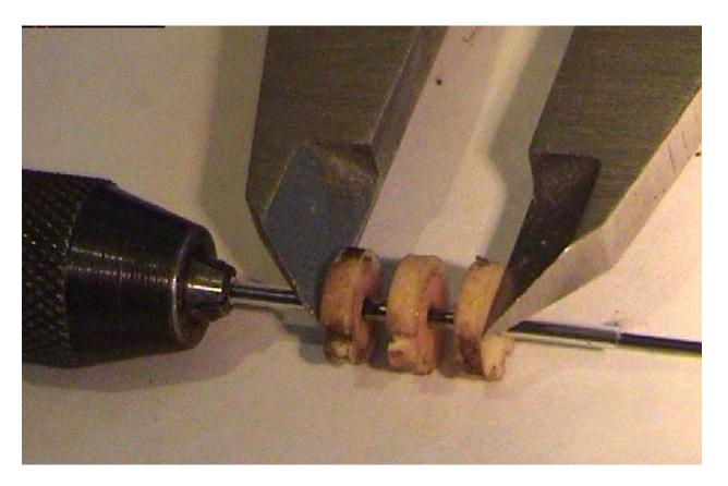
Here you see the three cheek pieces threaded onto the PTFE sleeving. There is a length of blue pivot steel inserted into the sleeving. The pin vice is gripping the sleeving in order to drive it. Note that the outside distance of the outer cheeks should be about 9.8mm. The centre cheek is centrally disposed between them.
