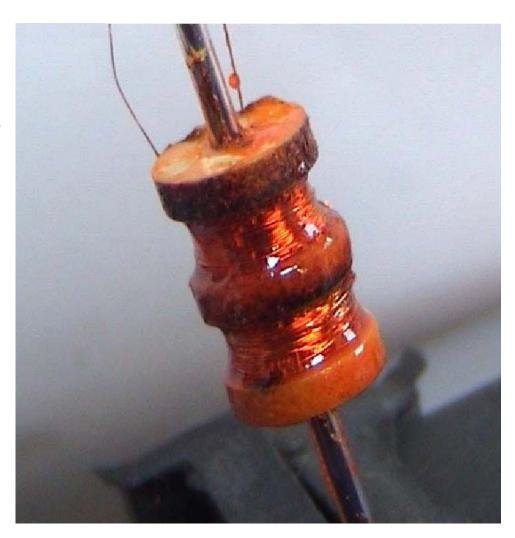
Carefully remove the central steel pin from the mandrel. Then ease the sleeving out of the coil assembly. Tin the wires and measure the resistance. 50 to 60 ohms is good. Infinity is disappointing.
