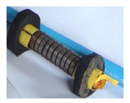
Place a doughnut over each copper cup, taking care not to damage the wires.
