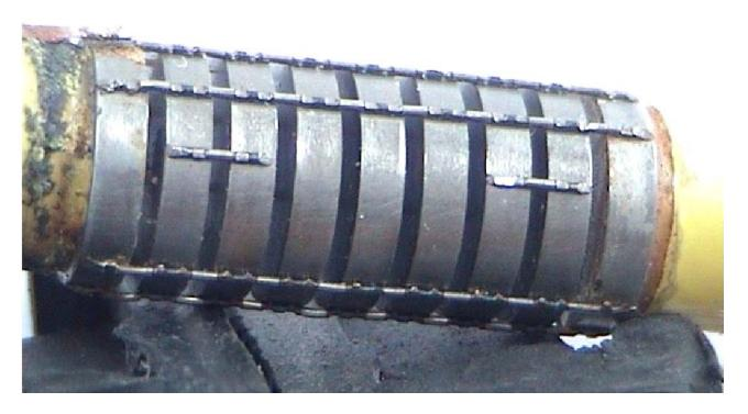
You will see that the filter comprises a set of disks with a coil at each end. This assembly will almost certainly need to be cleaned. In my case the debris from the foam had gone between the disks. Fortunately it seems to clean off quite well in alcohol.
