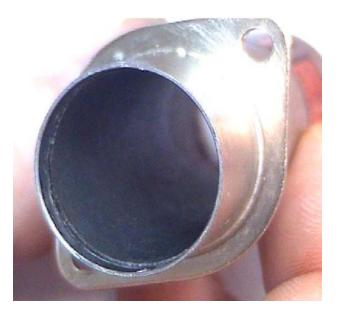
Make sure that the end caps are spotlessly clean, especially around the insulators. I placed a layer of Kapton tape over the internal surface. This was just a precaution to protect the fine wires from heat when re-soldering the case.
