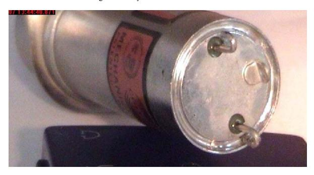
I am quite please with the appearance of the re-soldered caps. I think I got lucky! When I dismantled the 16 kHz filter, there was a load resistor fitted internally. It was wired in parallel with the coil at the output (top) end. The markings had all but gone but I think it was originally 56k. I elected not to refit this. This gave me the option of fitting an external resistor in order to balance my filter gains should the need arise. The 8 kHz did not have a resistor.
