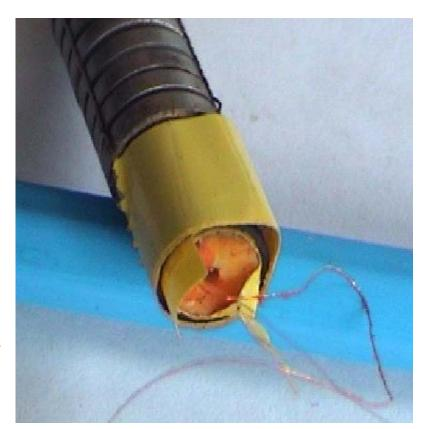
When you are happy with both coils, fifty to sixty ohms and no leakage to the metalwork, it is time to consider reassembly. You will need to replace the supporting doughnuts.
