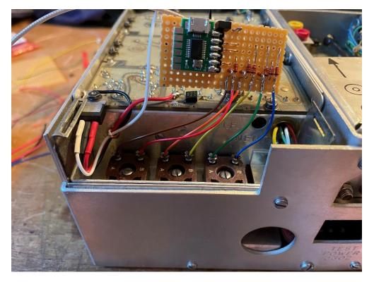
Connect the 5 volt line from the regulator and an additional ground wire from the Progrock ground to the ground trace on the front end board. This is the black wire shown below near the red power lead.
