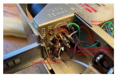
You will need to apply the ProgRock output to the grid connection that the green wire was removed from. I used miniature coax and grounded the coax shield to the bottom ground lug. Don't forget that the transmitter ProgRock module should have a capacitor on the output to the driver. You could mount this cap at the tube socket. I chose to mount it on the board with the ProgRock.
