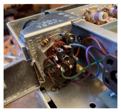
The picture below shows the wire attached to its new location on the ground lug.
