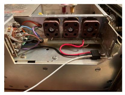
Now, you can connect the channel select lines to the crystal sockets. Be sure to use the top side of the crystal socket as shown in the photo below.
