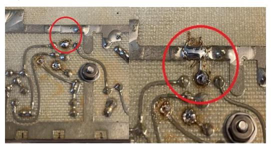
On the bottom of the board, you can see the original pad that was used for the switch connection is now used for the signal injection point into the oscillator circuit. The shield of the miniature coaxial cable is connected to the same point that the switch has been grounded to.
