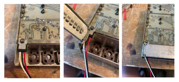
Attach the 12 volt input and ground leads to the points shown below. Be sure to install the 0.1 uF capacitor between the 12 volt point and ground as well. Ensure that the wires are dressed up away from the crystal sockets. There should be plenty of clearance underneath the regulator for the wires.
