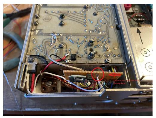
Connect the coax from the Progrock to the point shown below. This is the connection that was used previously by the channel switch. The cable can be grounded to the nearest ground trace.
