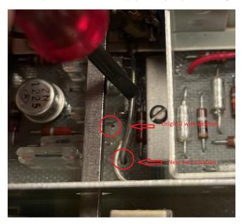
Pictured below is an example of a board without the complete ground trace. Note the jumper added to complete the connection.
