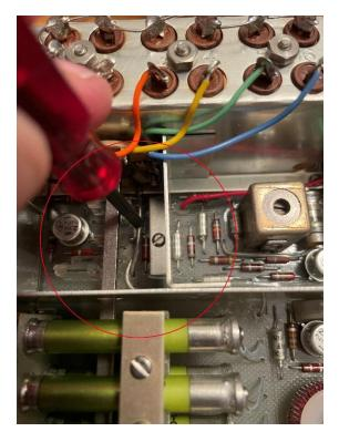
There is a lead running from the common switch terminal to the front end board as shown below. We are going to move this lead from its original location in the receiver LO to a nearby ground.
