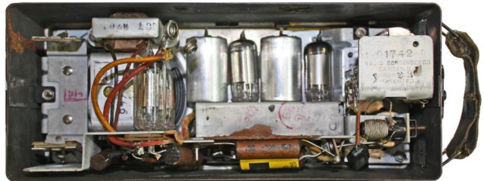
Internal view of the RCA Victor Model BP-10 with back cover removed. The 1.5V LT 'A' battery was carried on the left hand side and the 67.5V HT 'B' battery in the centre of the chassis.
