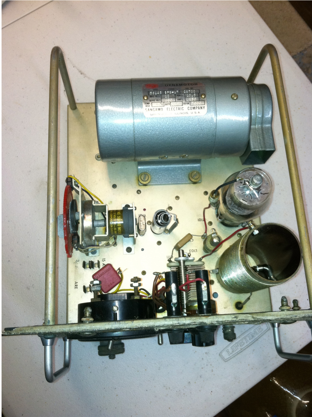
The transmitter and its dynamotor
