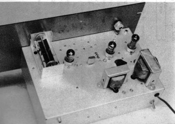
Fig. 5-33—Top view of the SimpleX Super. The tube at the left is the mixer-oscillator 6U8A; the 6CG7 audio amplifier is at the far right. The black knob is on the regeneration control. Toggle switch under the a.c. line cord is the a.c. line switch, S_3 . Phono jack at left is the antenna terminal; phono jack at right near volume control is speaker jack, J_s .
