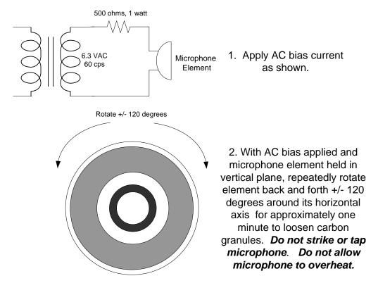
3. Maintaining AC bias and with microphone element held vertically, "blast" microphone diaphragm with acoustic white noise for 1-2 minutes to further loosen carbon granules. Receiver noise from handheld radio transceiver speaker closely coupled to diaphragm may be used as a noise source. If audio noise source is unavailable, blowing against microphone diaphragm may be used as an expedient.
