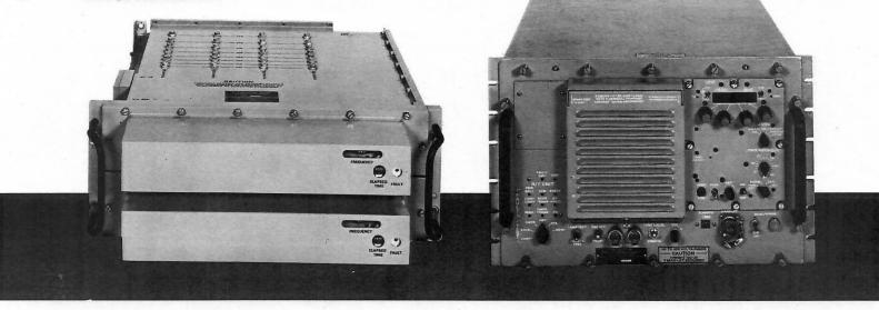
Collins Telecommunications Products Division, Rockwell International, has developed and is producing the AN/URC-93(V) (SATCOM — LOS VOICE — DATA LINK — ECCM) under contract to the US Navy. Navy Growth Radio is a versatile family of uhf radios and filters operating on 7,000 channels (25-kHz channel spacing) in the 225- to 400-MHz frequency range. This US Navy transceiver group presently consists of four shipboard versions and two airborne versions for voice, data, and wide-band communications.
