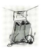
modes of operation. Calibration curves are mounted inside of the lid to aid in tuning. The batteries employed consist of three Z-30PX 45 volt B batteries, two 4FH A batteries and one 5540 C battery (Burgess).
