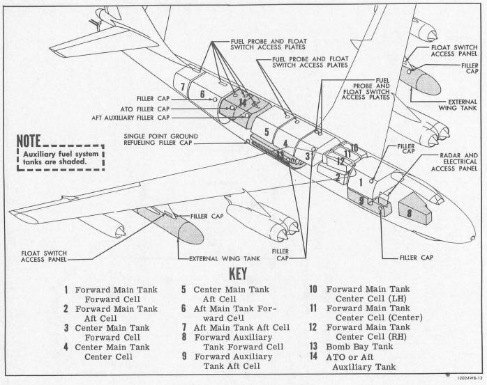
Figure 4-214. Fuel System Tanks
