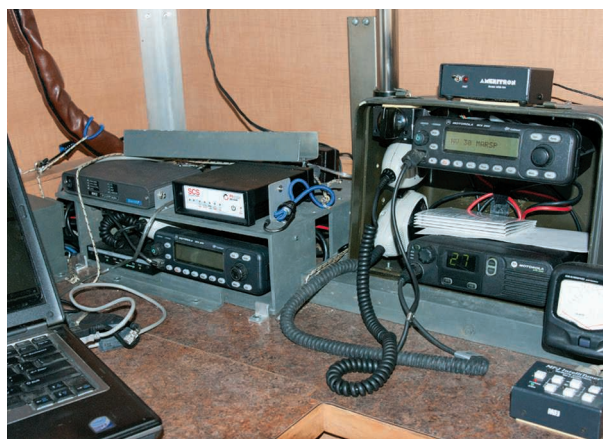
FIGURE 8. Three of the modems are shown. These include the SCS Pactor 3/4 modem, the RapidM RM2 modem for the military M110A mode, and the Kantronics Packet Modem. A modem for Winmor is behind the computer.
