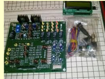
µBITX HF transceiver kit CW/SSB 10 watts http://www.hfsignals.com/
