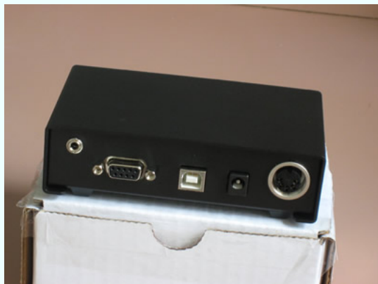
Connectors (Left to Right): Auxilliary Serial port, Serial Port, USB Port, External Power, Radio Connector
