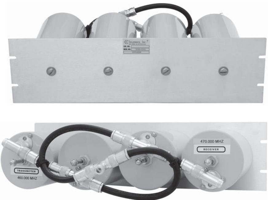
TPRD-4544/4744 duplexers mount on a 19" standard rack, with panel height of 5.25". Power handling is 250 watts. Receiver desense protection is at least 90 dB, and TX sideband suppression is at least 75 dB.
