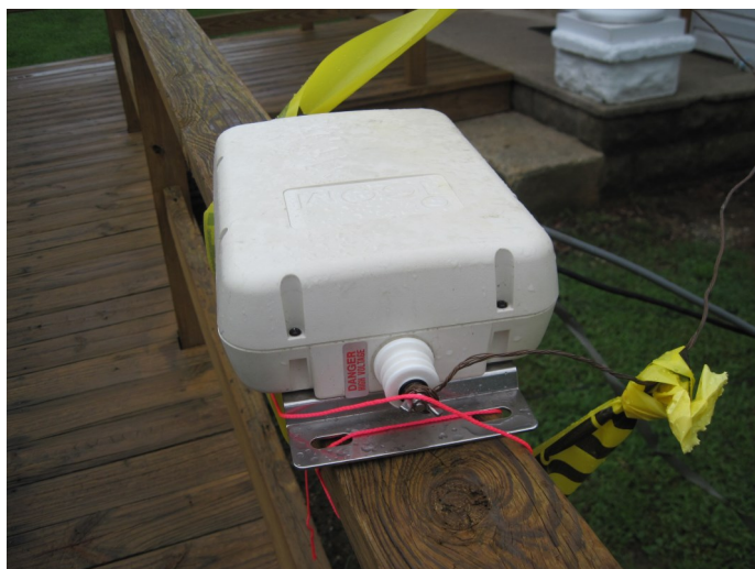
Ron's, WA4PRR; tuner for his long wire antenna. The rest of the wire was strung out to the edge of the street in front of the Community Center. We don't need no stinkin' tower!!
