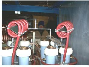
capable of output much higher than 125 KW. Very high RF currents, even in the water cooled copper tubing, lead to losses. Even if the tube itself is running at about 77% output, coupling losses occur as these units are usually inductively coupled to the load to be heated. Despite the losses the 125KW inductive heater with the BW1185J2 triode is one hefty RF power amplifier.
