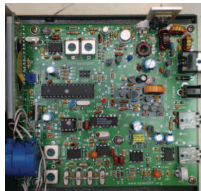
Figure 6 This low-cost, low-power continuous-wave transceiver uses a classic analog radio with a flexible programmable-control interface.
