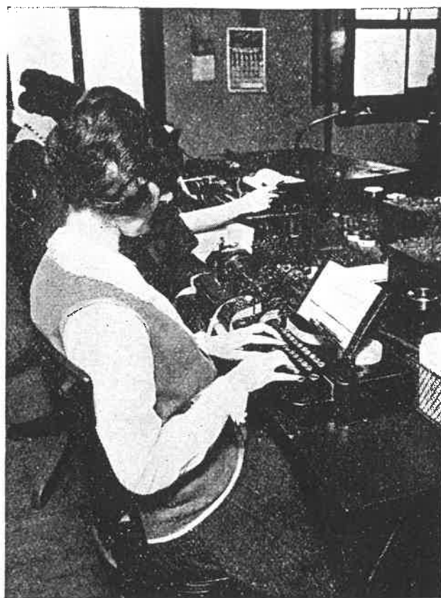
The sending keyboard of the duplex telegraph printer is almost exactly like that of a typewriter and the operation of transmission is closely akin to typing on an ordinary writing machine.
