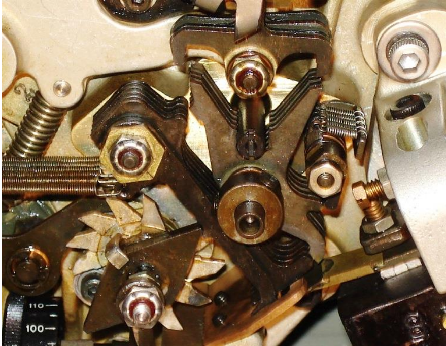
Left-to-Right: Printer Selector Levers, Y levers, and Y Detent Levers. The T-levers are above the Y-levers.
