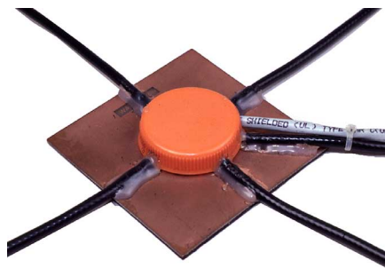
Antenna switcher close-up
