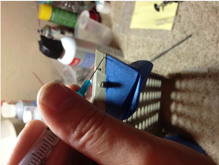
Applying ABS solvent to KB cover.
