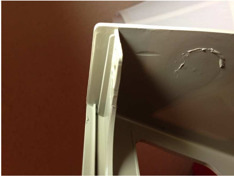
Side view of part after solvent welding.
