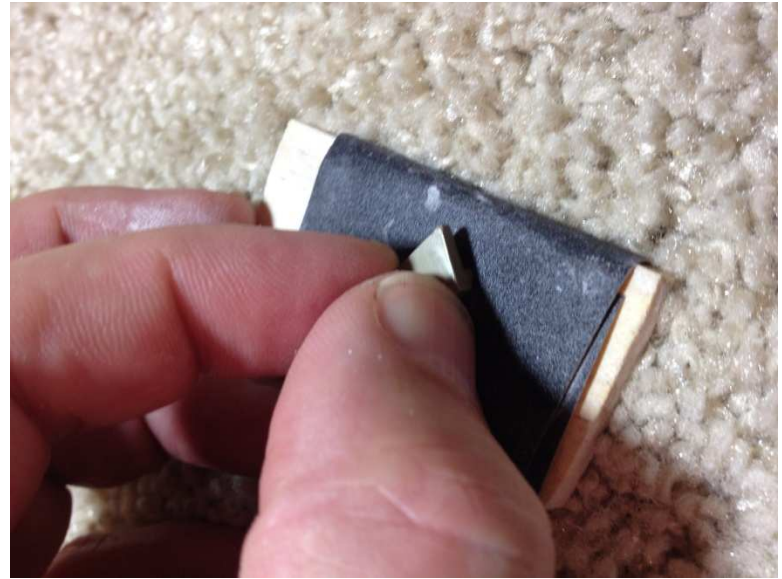
Forming replacement "ear" for keyboard cover using scrap plastic obtained from broken Teletype cover part.
