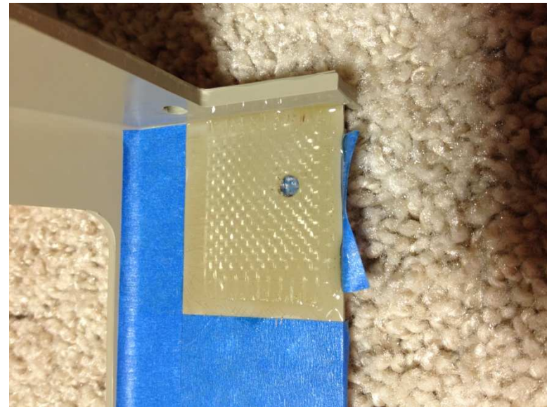
Resin applied over fiberglass patch.
