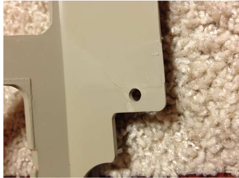
Solvent weld along full-thickness crack in plastic.
