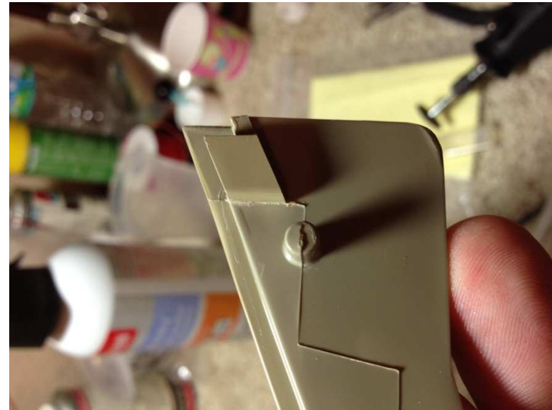
Cosmetics of the “ear” repair after solvent welding. NOTE: repair appears to be exceptionally strong and would be difficult to spot.
