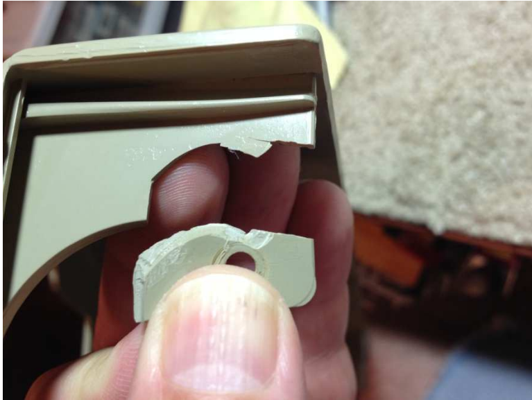
Example of damage to front part of cover.
