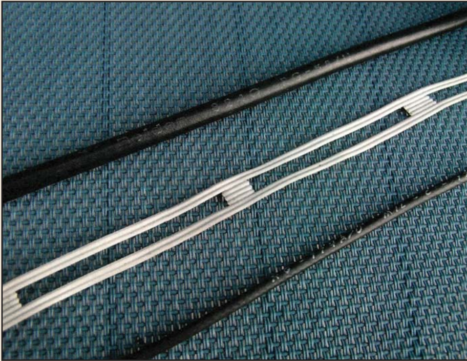
Photo D- Balanced feedline made from flat ribbon cable, flanked by RG-58 and RG-174.
