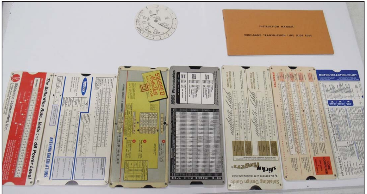
Photo B. Examples of specialized slide rules geared to various companies’ specific products. These were usually giveaways.
