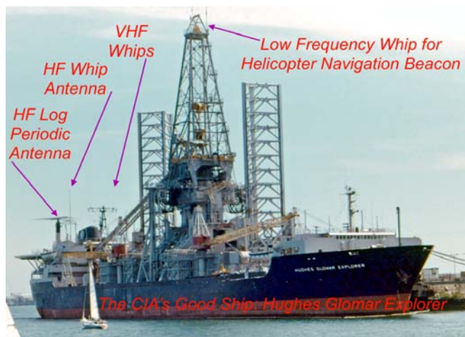
Fig. 2: Hughes Glomar Explorer , WCHG. Note antennas. The top right antenna on the derrick tower is the MF Beacon antenna for helicopter navigation to the ship.
