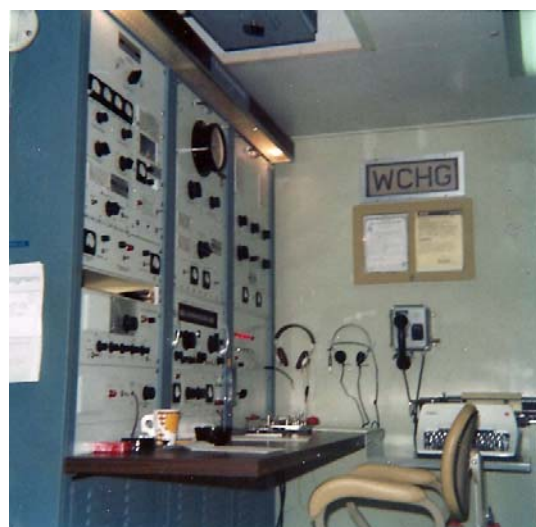
Fig. 5: Hughes Glomar Explorer WCHG transmitters: Collins 208U-3 (3 KW), and Communications Associates Inc. Transceiver (1 KW).
