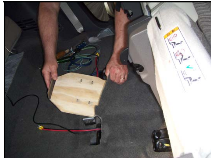
Under center of seat, after slitting carpet, padding is removed and used for a pattern for 1/4" plywood mount backed with an aluminum panel which is tied into car ground and the radio ground bar.
