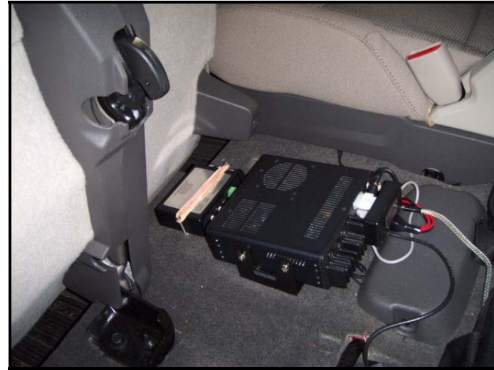
Radio after installation with tuner (left), all wiring is hidden and run under the carpet
