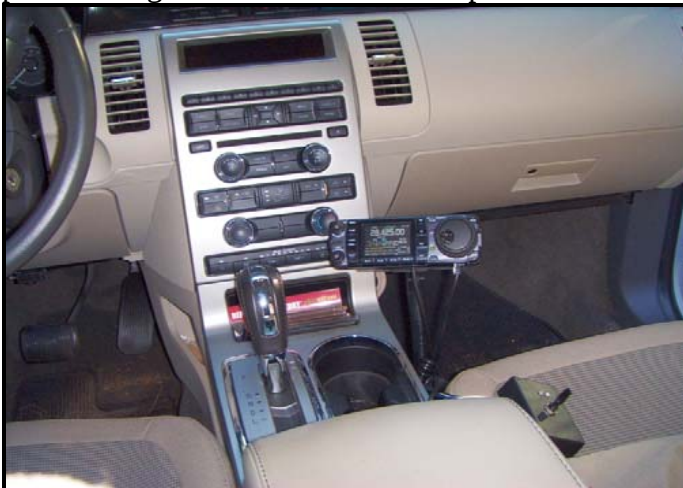
IC-7000 front panel mounted to flexible mount which is secured to front seat bolt
