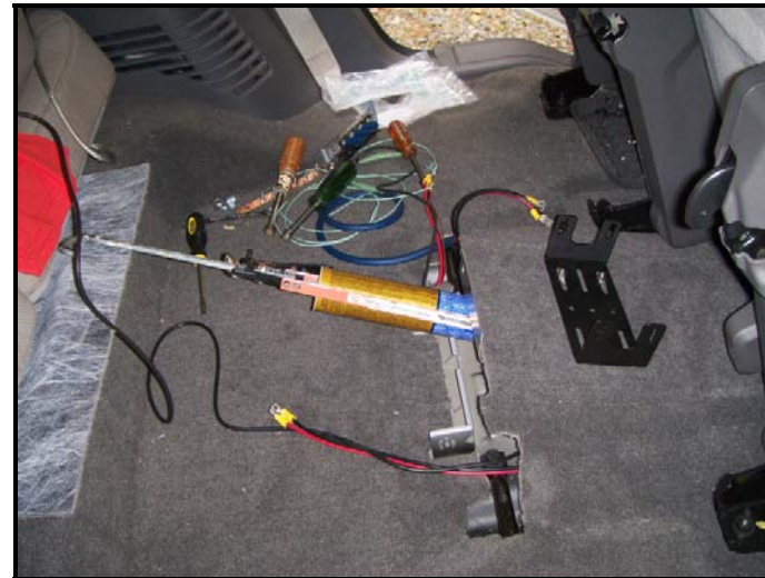
Plywood mount is glued down with industrial glue, no screws into metal floor due to gas tank under
