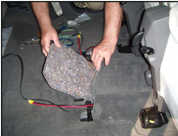
Under center of seat, after slitting carpet, padding is removed and used for a pattern for 1/4" plywood mount backed with an aluminum panel which is tied into car ground and the radio ground bar.
