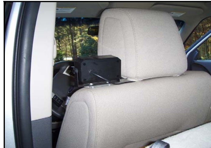
Speaker is mounted behind drivers left ear using Plexiglas secured under head rest supports, wiring routed through seat and under carpet to radio
