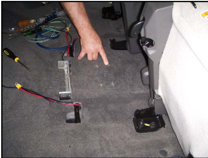
Carpet is slit for bolts to come through for mounting bracket
