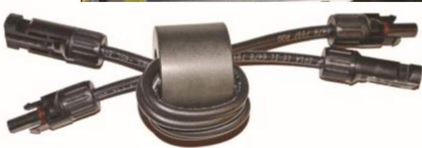
Figure 5 — Three bifilar turns of #10 PV wire on Fair-Rite 2631626202 core with MC4 connectors installed.
