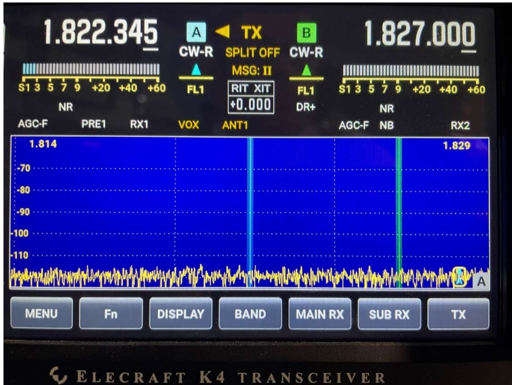
Figure 1 – Typical -120 dBm Noise Floor at the Station
